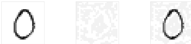
Fig. 1. (Left) Image from MNIST [16] dataset, which is correctly classified as 0 by a given neural network. (Center) A small perturbation applied to the image. (Right) Resulting noisy image classified by the same neural network as a 3 with 92% confidence.
